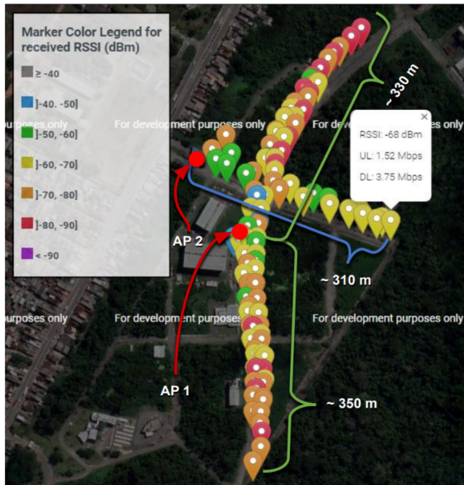
Figure 4.15: Results of the network validation experiment in a controlled environment.
